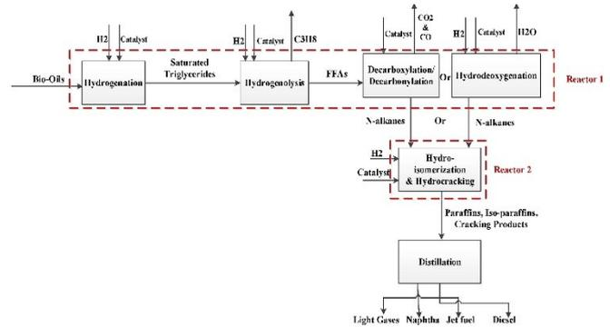
Fig. 3. Diagram of the HRJ Conversion Technology's Workflow [17].
