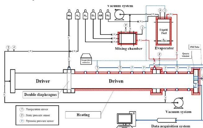
Figure 4. Schematic Diagram of Shock Tube [21].
