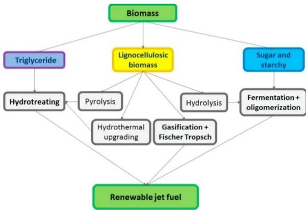
Fig. 1. Production Routes for Bio-Jet Fuel [12].
